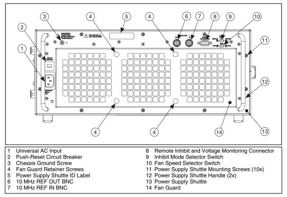
Figure 1-2. Rear View of the NI PXIe-1065 Chassis
